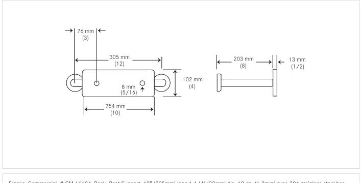
Franke Commercial # CM-16104 Back Rest Support, 12" (305mm) long 1-1/4" (32mm) dia. 18 ga. (1.3mm) type 304 stainless steel bar with flanges and covers and with 10" x 4" (254mm x 102mm) antique white plastic laminate face on solid black phenolic core and secured with stainless steel screws. Projection from wall – 8-1/2" (216mm). Provide adequate backing in wall for support and comply to local codes for barrier free requirements.
