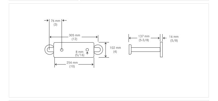
Franke Commercial 'MIDLAND' #CM-16104-WM Back Rest Support for wall mounted toilets, 12" (305mm) long x 1-1/4" (32mm) dia. 18 ga. (1.3mm) type 304 stainless steel bar with flanges and covers and with 10" x 4" (254mm x 102mm) antique white plastic laminate face on solid black phenolic core and secured with stainless steel screws. Projection from wall – 6" (153mm). Provide adequate backing in wall for support and comply to local codes for barrier-free requirements.
