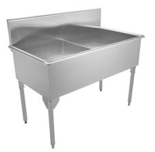
Double compartment scullery sink. 16 gauge (1.5 mm), type 304 (CNS 18/10) stainless steel. Polished to a #4 satin finish. Sink compartments sloped to drain with radius coved corners on front and back only. Rolled rim. Stainless steel tubular legs with adjustable feet. Includes waste fittings. Certified to ASME A112.19.3-2008 / CSA B45.4-08
