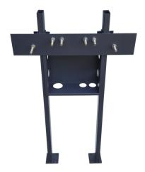
Floor mounted in-wall carrier designed for Medi-flo (HWSS23221W) Hand Hygiene Sink. Preset stud locations simplify installation. Steel uprights with welded feet. Integrated rough in box. Mounting hardware included.
