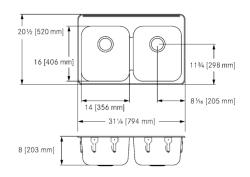
Double compartment self rimming topmount sink with faucet ledge. 18 gauge (1.2 mm), type 304 (CNS 18/10),18-10 stainless steel. Exposed surfaces are #4 satin finished. Undercoated to reduce condensation and resonance. Includes waste fittings, factory applied rim seal, cutout template, and factory installed EZ TORQUE™ fasteners. Certified to ASME A112.19.3-2008 / CSA B45.4-08.
