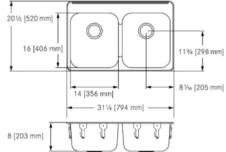
Double compartment self rimming topmount sink with faucet ledge. 20 gauge (0.9 mm), type 302 (CNS 18/8) stainless steel. Exposed surfaces are #4 satin finished. Spillway® between bowls. Undercoated to reduce condensation and resonance. Includes waste fittings, factory applied rim seal, cutout template, and factory installed EZ TORQUE™ fasteners. Certified to ASME A112.19.3-2008 / CSA B45.4-08.
