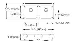
Double compartment self rimming topmount sink with faucet ledge. 20 gauge (0.9 mm), type 302 (CNS 18/8) stainless steel. Exposed surfaces are #4 satin finished. Spillway® between bowls. Undercoated to reduce condensation and resonance. Includes waste fittings, factory applied rim seal, cutout template, and factory installed EZ TORQUE™ fasteners. Certified to ASME A112.19.3-2008 / CSA B45.4-08.
