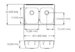
Double compartment self rimming topmount sink with faucet ledge. 20 gauge (0.9 mm), type 302 (CNS 18/8) stainless steel. Exposed surfaces are #4 satin finished. Spillway® between bowls. Undercoated to reduce condensation and resonance. Includes waste fittings, factory applied rim seal, cutout template, and factory installed EZ TORQUE™ fasteners. Certified to ASME A112.19.3-2008 / CSA B45.4-08.
