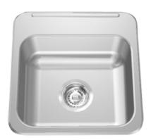
Single compartment self rimming topmount sink with faucet ledge. 20 gauge (0.9 mm), type 302 (CNS 18/8) stainless steel. Exposed surfaces are #4 satin finished. Undercoated to reduce condensation and resonance. Includes waste fitting, factory applied rim seal, cutout template, and factory installed EZ TORQUE™ fasteners. Certified to ASME A112.19.3-2008 / CSA B45.4-08.
