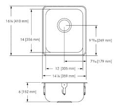
Single compartment self rimming topmount sink less faucet ledge. 20 gauge (0.9 mm), type 302 (CNS 18/8) stainless steel. Exposed surfaces are #4 satin finished. Undercoated to reduce condensation and resonance. Includes waste fitting, factory applied rim seal, cutout template, and factory installed EZ TORQUE™ fasteners. Certified to ASME A112.19.3-2008 / CSA B45.4-08.
