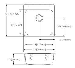
Single compartment self rimming topmount sink with faucet ledge. 20 gauge (0.9 mm), type 302 (CNS 18/8) stainless steel. Exposed surfaces are #4 satin finished. Undercoated to reduce condensation and resonance. Includes waste fitting, factory applied rim seal, cutout template, and factory installed EZ TORQUE™ fasteners. Certified to ASME A112.19.3-2008 / CSA B45.4-08.
