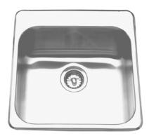
Single compartment self rimming topmount sink with faucet ledge. 18 gauge (1.2 mm), type 304 (CNS 18/10) stainless steel. Exposed surfaces are #4 satin finished. Undercoated to reduce condensation and resonance. Includes waste fitting, factory applied rim seal, cutout template, and factory installed EZ TORQUE™ fasteners. Certified to ASME A112.19.3-2008 / CSA B45.4-08.
