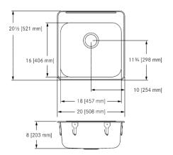
Single compartment self rimming topmount sink with faucet ledge. 20 gauge (0.9 mm), type 302 (CNS 18/8) stainless steel. Exposed surfaces are #4 satin finished. Undercoated to reduce condensation and resonance. Includes factory applied rim seal, cutout template, and factory installed EZ TORQUE™ fasteners. Certified to ASME A112.19.3-2008 / CSA B45.4-08 Centre back waste location. Includes 3 1/2" (89 mm) crumb cup strainer with 1 1/2" (DN38) brass tailpiece. Model Options:
