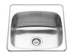
Single compartment self rimming topmount sink with faucet ledge. 18 gauge (1.2 mm), type 304 (CNS 18/10) stainless steel. Exposed surfaces are #4 satin finished. Undercoated to reduce condensation and resonance. Includes waste fitting, factory applied rim seal, cutout template, and factory installed EZ TORQUE™ fasteners. Certified to ASME A112.19.3-2008 / CSA B45.4-08.
