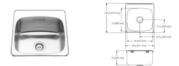
Single compartment self rimming topmount sink with faucet ledge. 18 gauge (1.2 mm), type 316 (EN 1.4401 17/12/2) stainless steel. Exposed surfaces are #4 satin finished. Undercoated to reduce condensation and resonance. Includes waste fitting, factory applied rim seal, cutout template, and factory installed EZ TORQUE™ fasteners. Certified to ASME A112.19.3-2008 / CSA B45.4-08.
