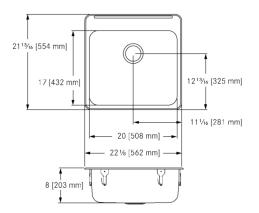
Single compartment self rimming topmount sink with faucet ledge. 18 gauge (1.2 mm), type 304 (CNS 18/10) stainless steel. Exposed surfaces are #4 satin finished. Undercoated to reduce condensation and resonance. Includes waste fitting, factory applied rim seal, cutout template, and factory installed EZ TORQUE™ fasteners. Certified to ASME A112.19.3-2008 / CSA B45.4-08.
