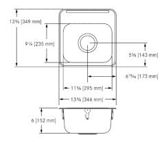
Single compartment self rimming topmount sink with faucet ledge. 20 gauge (0.9 mm), type 302 (CNS 18/8) stainless steel. Exposed surfaces are #4 satin finished. Undercoated to reduce condensation and resonance. Includes waste fitting, factory applied rim seal, cutout template, and factory installed EZ TORQUE™ fasteners. Certified to ASME A112.19.3-2008 / CSA B45.4-08.
