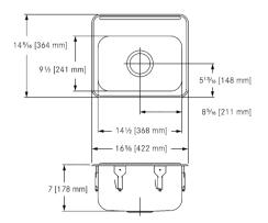
Single compartment self rimming topmount sink with faucet ledge. 18 gauge (1.2 mm), type 316 (EN1.4401 17/12/2) stainless steel. Exposed surfaces are #4 satin finished. Undercoated to reduce condensation and resonance. Includes waste fitting, factory applied rim seal, cutout template, and factory installed EZ TORQUE™ fasteners. Certified to ASME A112.19.3-2008 / CSA B45.4-08.
