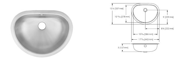
Single compartment undermount vanity basin. 18 gauge (1.2 mm), type 304 (CNS 18/10) stainless steel. Exposed surfaces are #4 satin finished. Undercoated to reduce condensation and resonance. Includes cutout template and installation hardware. Certified to ASME A112.19.3-2008 / CSA B45.4-08.
