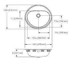
Single compartment self rimming vanity basin with faucet ledge. 18 gauge (1.2 mm), type 304 (CNS 18/10) stainless steel. Mirror finished rim, #4 satin finished bowl. Undercoated to reduce condensation and resonance. Includes factory applied rim seal, cutout template, and installation hardware. Certified to ASME A112.19.3-2008 / CSA B45.4-08.
