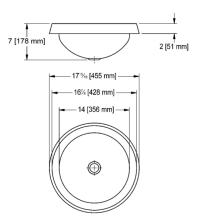
Single compartment semi-recessed vanity basin less faucet ledge. 18 gauge (1.2 mm), type 304 (CNS 18/10) stainless steel. Mirror finished rim, #4 satin finished bowl. Undercoated to reduce condensation and resonance. Includes cutout template and installation hardware. Certified to ASME A112.19.3-2008 / CSA B45.4-08.
