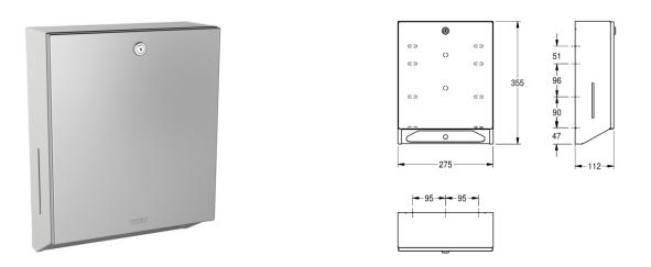
Paper towel dispenser for wall mounting, stainless steel, surface satin finished, material thickness 0.8 mm, folded front cover, cylinder lock with Franke standard key, inspection windows on sides, loading capacity 300 - 400 pcs. of paper depending on convolution, includes stainless steel screws and dowels.
