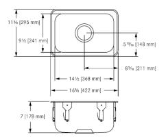
Single compartment self rimming topmount sink less faucet ledge. 20 gauge (0.9 mm), type 302 (CNS 18/8) stainless steel. Exposed surfaces are #4 satin finished. Undercoated to reduce condensation and resonance. Includes waste fitting, factory applied rim seal, cutout template, and factory installed EZ TORQUE™ fasteners. Certified to ASME A112.19.3-2008 / CSA B45.4-08.
