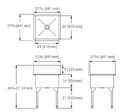
Single compartment scullery sink. 16 gauge (1.5 mm), type 304 (CNS 18/10) stainless steel. Polished to a #4 satin finish. Sink compartment sloped to drain with radius coved corners on front and back only. Rolled rim. Stainless steel tubular legs with adjustable feet. Includes waste fitting. Certified to ASME A112.19.3-2008 / CSA B45.4-08 Centre waste location. Includes 3 1/2" (89 mm) crumb cup strainer with 1 1/2" (DN38) brass tailpiece. Model Options:
