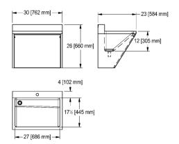
Single compartment surgical scrub station. 18 gauge (1.2 mm), type 304 (CNS 18/10) stainless steel. Polished #4 satin finish. Radius coved bowl corners. Franke hygienic waste with integral talipiece. (No separate waste fitting required) Access panel for service and maintenance. Supplied with wall hanger brackets. Certified to ASME A112.19.3-2008 / CSA B45.4-08. Faucet not included with base model, see below for options. Please specify hole drilling requirement when ordering.
