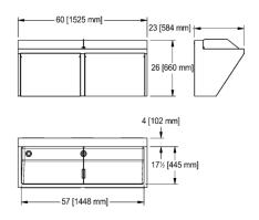
Double compartment surgical scrub station. 18 gauge (1.2 mm), type 304 (CNS 18/10) stainless steel. Polished #4 satin finish. Radius coved bowl corners. Franke hygienic waste with integral talipiece. (No separate waste fitting required) Access panel for service and maintenance. Removable divider. Supplied with wall hanger brackets. Please specify
