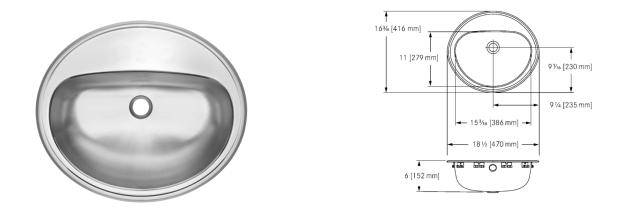
Single compartment self rimming vanity basin with faucet ledge. 18 gauge (1.2 mm), type 304 (CNS 18/10) stainless steel. Mirror finished rim, #4 satin finished bowl. Undercoated to reduce condensation and resonance. Includes factory applied rim seal, cutout template, and installation hardware. Certified to ASME A112.19.3-2008 / CSA B45.4-08.
