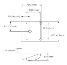
Wall hung basin. Centre back waste location. 18 gauge (1.2 mm), type 304 (CNS 18/10) stainless steel. Exposed surfaces are #4 satin finished. Radius coved bowl corners. One piece wall hanger. Waste assembly included. Certified to ASME A112.19.3-2008 / CSA B45.4-08.
