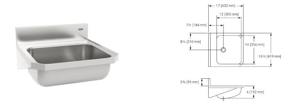
Wall hung basin. Centre back waste location. 18 gauge (1.2 mm), type 304 (CNS 18/10) stainless steel. Exposed surfaces are #4 satin finished. Radius coved bowl corners. One piece wall hanger. Waste assembly is not included. Certified to ASME A112.19.3-2008 / CSA B45.4-08. Separate sink carrier is not required.
