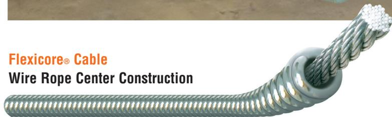
Heavy-gauge wire coiled tightly around 49-strand aircraft-type wire rope and heat treated. Has unequalled strength and the right amount of flexibility. So tough it carries a one-year warranty against defect or breakage.
