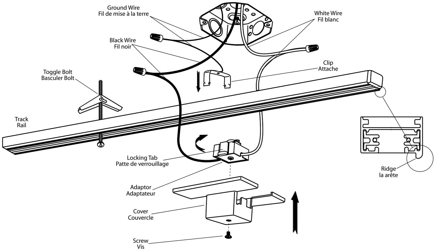
1. Insert the adaptor with the polarity groove towards the polarity ridge on the track (The locking tab on the opposite side of the track ridge).
