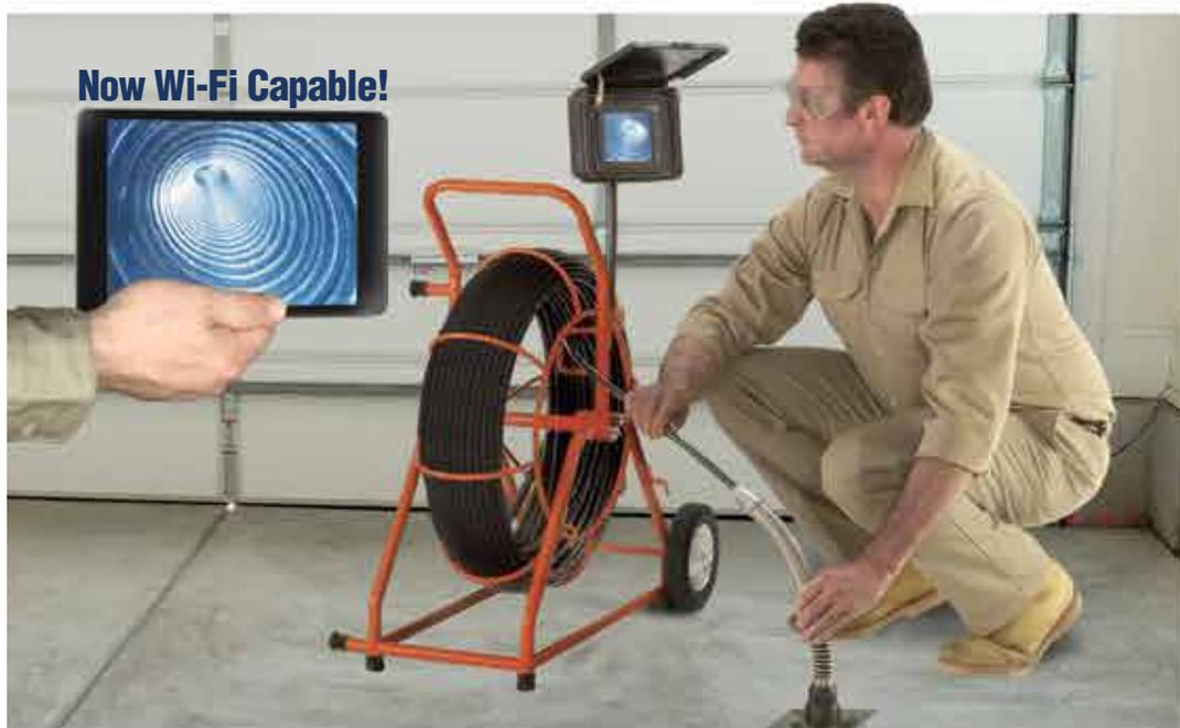
There's lots more, like the LED Dimmer Control, both AC and DC power cords, 2", 3" and 6" Trap Skids, and a 512 Hz transmitter. A video out connection lets you record on an external device.
