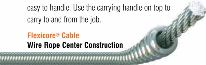
Heavy-gauge wire coiled tightly around 49-strand aircraft-type wire rope and heat treated. Has unequalled strength and the right amount of flexibility. So tough it carries a one-year warranty against defect or breakage.
