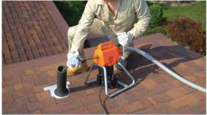
The Root 66 has a wide four point base for greater stability. Its interlocking tubular construction also gives it excellent durability. To protect the gears from dirt and for easier cleaning, the machine has two internal plastic shields. A Ground Fault Circuit Interrupter is standard equipment.
