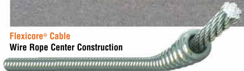
Heavy-gauge wire coiled tightly around 49-strand aircraft-type wire rope and heat treated. It has unequalled strength and the right amount of flexibility. So tough it carries a one-year warranty against defect or breakage.
