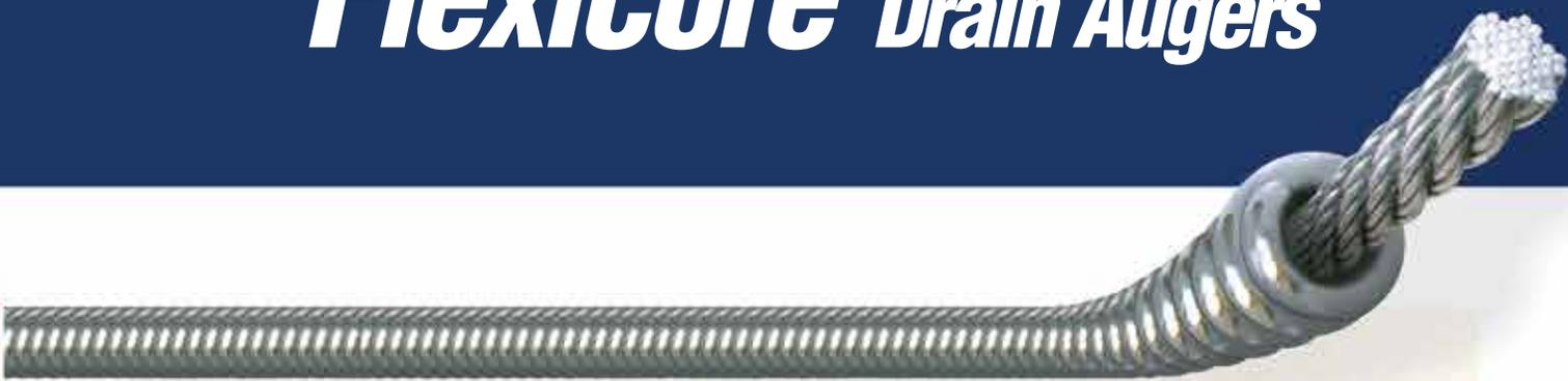
A core of aircraft-type wire rope makes Flexicore Augers so tough they carry a one-year warranty (see page 3). After coiling, they're heat treated for maximum toughness and durability. Right-hand wind makes manual operation easier through greater flexibility.
