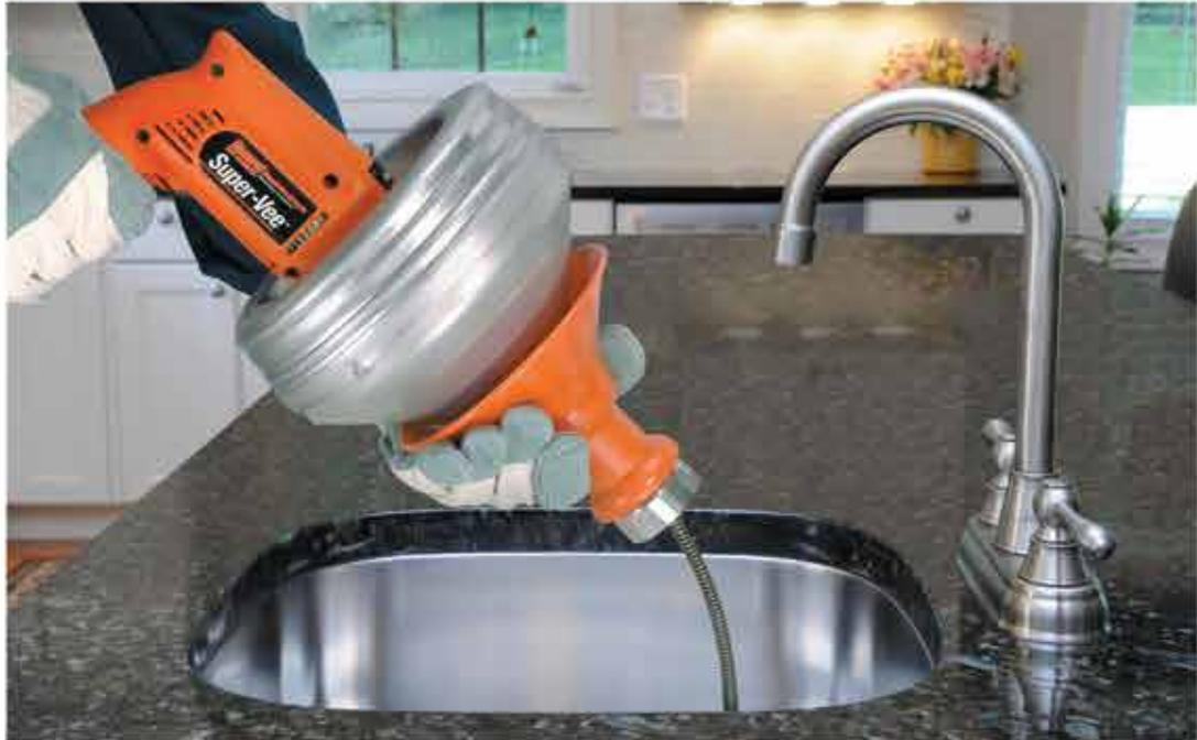
To switch to a different diameter cable you just loosen three screws, pull the front of the drum off the cable, and load in another cartridge. Changing takes less than a minute and turns what could be a messy job into a clean one. The tough plastic cartridges are so inexpensive, you'll probably want to store all of your cables in them.
