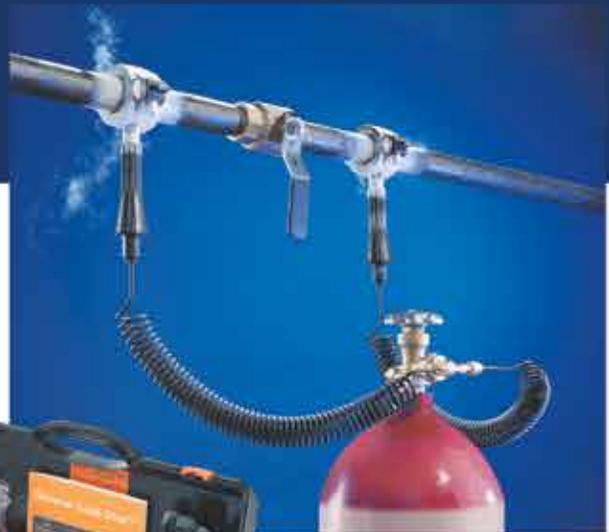
Kit includes 10 sets of freeze heads for 1/8" to 2" lines (10 mm to 60 mm), two high pressure spiral hoses with injectors, T-distributor, locking nut, hex head screwdriver, rubber gloves, goggles and carrying case.
