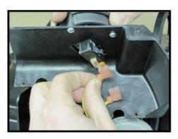
6. Cut a square opening in the electric box cover using a knife or a file.
