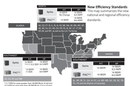
\*\*PAC includes both single package cooling only and single package gas/electric models
