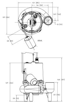
All dimensions in inches. Component dimensions may vary ± 1/8 inch. Dimensional data not for construction purpose unless certified. Dimensions and weights are approximate. On/Off level adjustable.
