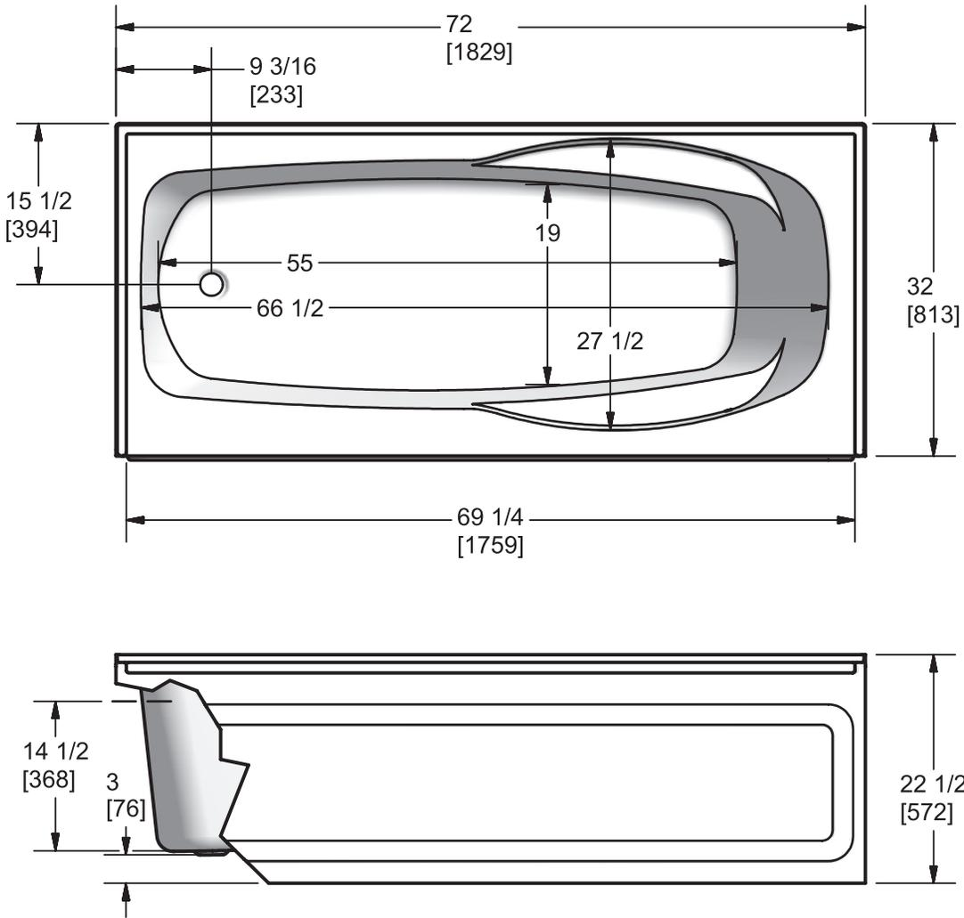
Measurement tolerances  $\pm 1/4"$  (6.3 mm)
