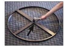
Screw center shaft into base with wrench.
