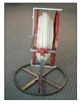
lifting at the front of the extension arm (at pipe guide). This allows the sliding movement of the square tubing left or right for balancing adjustment. Adjust the combined dispenser wheel with a loaded pipe roll until wheel is vertical and pipe will rotate freely in either direction. When final position chosen ensure both left and right hub sleeve bolts are tightened securely.
