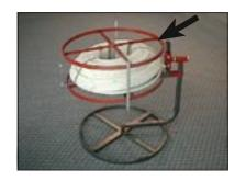
Place roll of pipe onto wheel. Lock pipe roll into position with retaining wheel.
