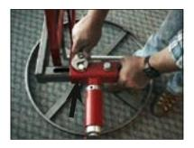
Temporarily tighten one hub sleeve bolt onto crosspiece arm.
