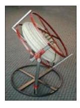
Loosen locking fork; pipe & dispenser wheel will now move freely but most likely will be positioned at a 45° angle. For optimum operation, dispenser wheel and pipe assembly should be properly balanced. This will allow for the easy removal of any "pipe twist" as the pipe is being uncoiled. To balance wheel, relieve weight off square tubing by
