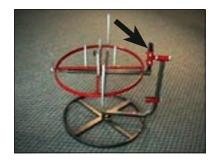
Install cross piece / rotating wheel with 1 1/2" square tubing (90° attached arm) and slide into bearing hub sleeve.
