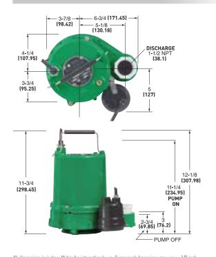
All dimensions in inches. Metric for international use. Component dimensions may vary ± 1/8 inch. Dimensional data not for construction purpose unless certified. Dimensions and weights are approximate. On/Off level adjustable.
