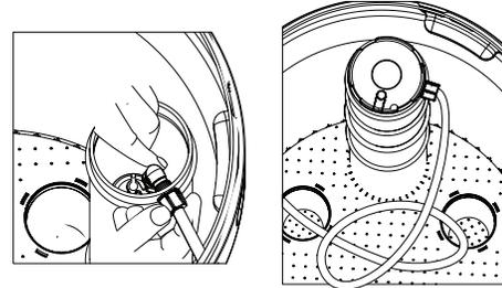
f. For installation of brine tank at the installation site, pull the other end of the brine tube from the hole on the brine tank. The completed assembly is shown below.
