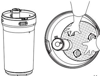
The hole in the brine tank should line up with the brine line as shown for round and square brine tank.
