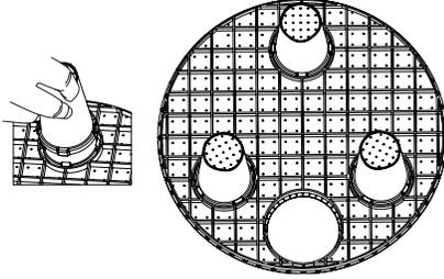
b. Insert the brine well assembly inside the grid plate as well below.
