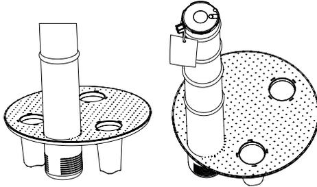
c. Drop the brine grid with brine well inside the brine tank such that the nut fitting faces the hole on the brine tank. Then press the grid evenly inside the brine tank until the brine grid legs touches the bottom of the brine tank.
