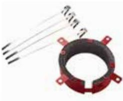
Ultra Plastic Pipe Device is red coloured, contains 3M™ Interam™ Ultra GS wrap material in a preformed collar. When exposed to temperatures of 121°C the wrap material expands (up to 25 times) to seal combustible pipe service penetrations.
