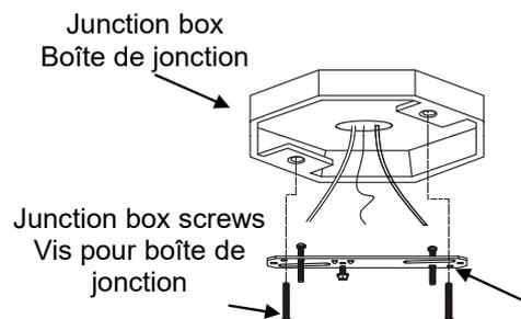
Attach the mounting bracket to junction box with screws provided.
