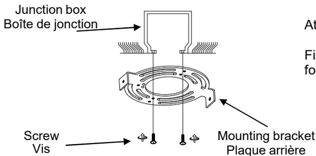
Attach the mounting bracket to junction box with screws provided.
