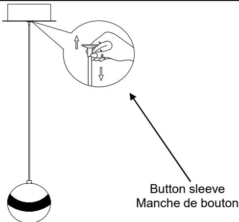
Before installation to ceiling, adjust fixtures to desired length by pushing wire up into canopy, then coiling up excess wire, minor adjustment can be made after installation. To lower or lengthen wire, depress button sleeve located where wire comes out of canopy.
