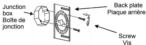
Attach the back plate to the junction box with screws provided.
