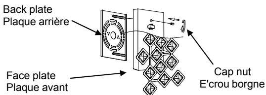
Attach the face plate to the back plate with cap nuts provided.
