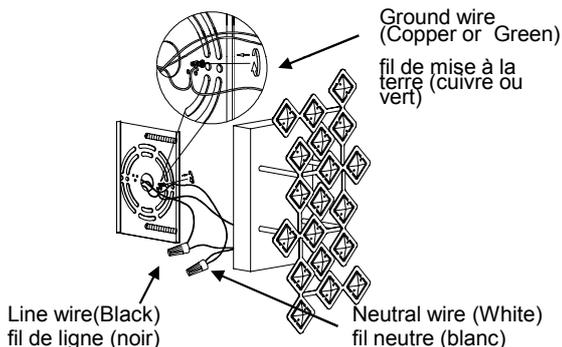
Connect the GROUND WIRE from junction box to GROUND (or GREEN) with a wire nut. Connect the NEUTRAL WIRE from junction box to NEUTRAL (WHITE) wire from fixture with a wire nut. Connect the LINE WIRE from junction box to LINE (BLACK) wire from fixture with a wire nut.
