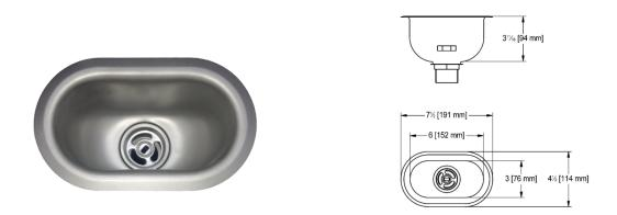
Single bowl commercial laboratory sink. 20 gauge (0.9 mm), type 316 (EN1.4401 17/12/2) stainless steel. Exposed surfaces are sand-blast finished. Positive hold down clamping. 1 1/2" (38 mm) type 316 (EN1.4401 17/12/2) stainless steel duplex waste assembly is integral (tailpiece optional\*). Certified to ASME A112.19.3-2008 / CSA B45.4-08. Centre waste location
