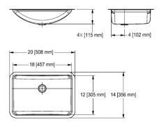
Single compartment undermount vanity basin. 18 gauge (1.2 mm), type 304 (CNS 18/10) stainless steel. Exposed surfaces are #4 satin finished. Undercoated to reduce condensation and resonance. Includes cutout template. Certified to ASME A112.19.3-2008 / CSA B45.4-08.
