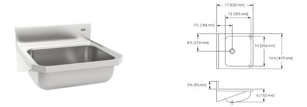
Wall hung basin. Centre back waste location. 18 gauge (1.2 mm), type 304 (CNS 18/10) stainless steel. Exposed surfaces are #4 satin finished. Radius coved bowl corners. One piece wall hanger. Waste assembly included. Certified to ASME A112.19.3-2008 / CSA B45.4-08.
