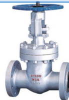
276-CS-600 , Globe Valve, Class 600, F-F Flanged Ends, Bolted Bonnet, 13Cr/HF Iron, WCB Body & Bonnet
