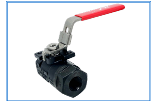
C-206TWL , 6000 WOG, NPT Ends 1/4" - 1 1/2" - Full Port, 2" - Standard Port
