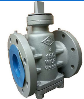
282-CS-150 , Balancing Plug Valve, Class 150, F-F Flanged Ends, Bolted Bonnet, 13Cr/HF Trim WCB Body & Bonnet
