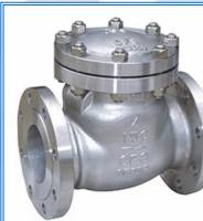
278-CS-150 , Swing Check Valve, Class 150, F-F Flanged Ends, Bolted Bonnet, 13Cr/HF Iron, WCB Body & Bonnet
