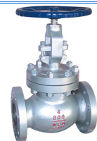
276-CS-300 , Globe Valve, Class 300, F-F Flanged Ends, Bolted Bonnet, 13Cr/HF Iron, WCB Body & Bonnet
