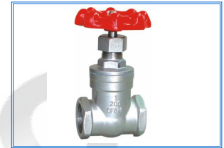
2GATS , 200 WOG, Non Rising Stem Gate Valve, NPT Ends
