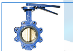
BL-1000-11DBL (DEL) 200 WOG, Buna(DB) or EPDM(DE) Seat, DI NP Disc
