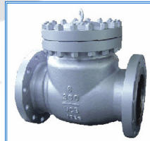
278-CS-300 , Swing Check Valve, Class 300, F-F Flanged Ends, Bolted Bonnet, 13Cr/HF Iron, WCB Body & Bonnet
