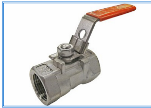
S-121T , 1000 WOG, 1-Piece Reduced Port, NPT Ends
