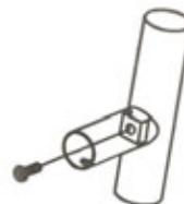
11. Secure assembled 'railing/wall spacers' to wall brackets.
