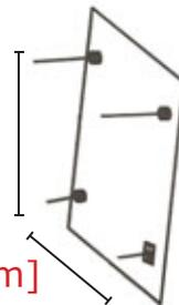
7. Mark pilot hole placement. Ensure installation points are square.
