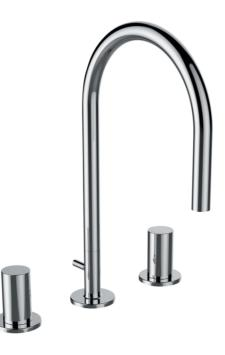
Acoustic Level (dB) : Group 1 (Up to 20 dB) Aerator type : Honeycomb PCA Application place : Basin Faucet type : Twin-lever Finish : Chrome Flexible supply hoses included Flow rate (I/min - 3 bar) : 5.7 Installation type : Deck-mounted Net weight (kg) : 2.25 Spout length (mm) : 166 Spout position : High Swivel spout Twin lever control : 1/4 Turn Type of cartridge : Ceramic
