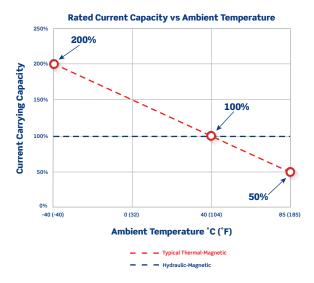
Hydraulic-Magnetic trip technology helps prevent false tripping, even in extreme temperature ranges<sup>1</sup>, unlike traditional Thermal-Magnetic circuit breakers
